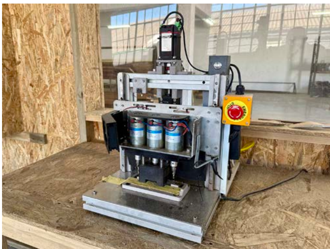
Donkey Long Tong's Head of Engineering, Luke Dyson, designed and built a drill press that could drill three little holes instead of a single drill press drilling out holes individually to speed up the production of their fire tool handles
