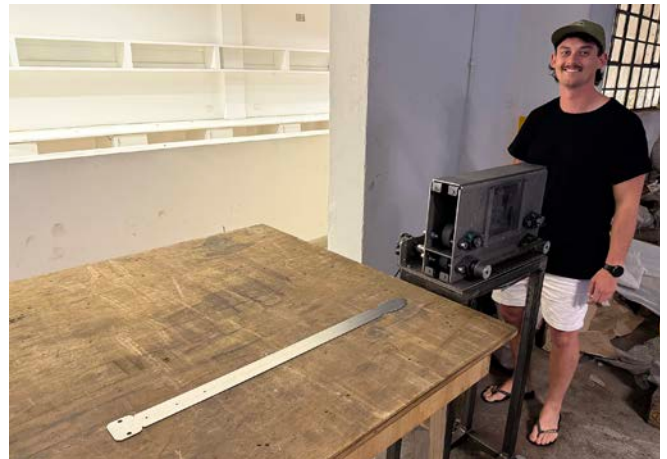
The 'tong gobbler' is a polishing wheel, and it gives Donkey Long Tong a certain surface finish that they are after when pre-cleaning their tong blanks. Luke Dyson, Donkey Long Tong's Head of Engineering and a mechanical engineer by trade, designed and built the machine along with one of Donkey Long Tong's cofounder's, Marcel
