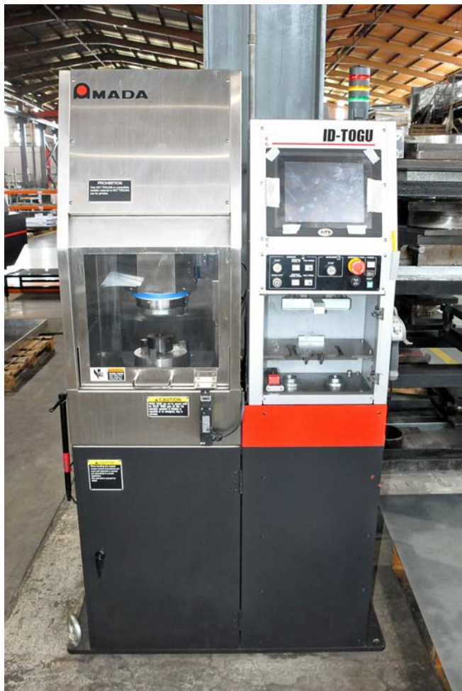
HC Heat Exchangers have installed an Amada ID-TOGU automatic tool grinding machine. Tooling maintenance is an important and indispensable element to keeping product quality in sheet metal products
