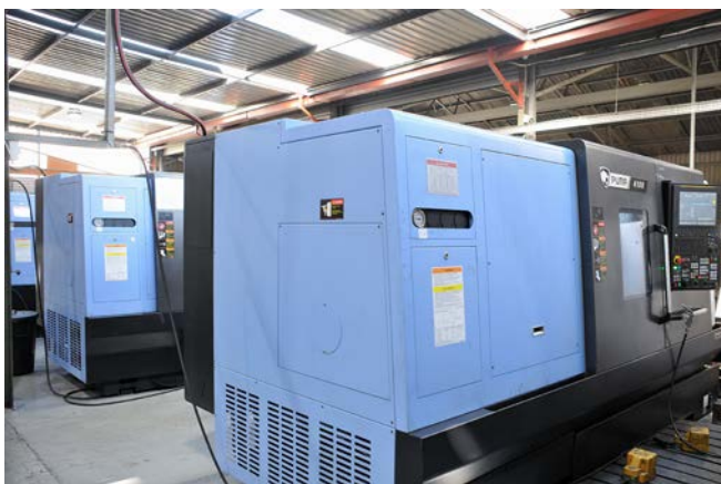
PTF have invested in a number of new DN Solutions Puma 4100 series turning centers, which is primarily aimed at precision component manufacturers machining large to medium parts for many different industrial sectors
