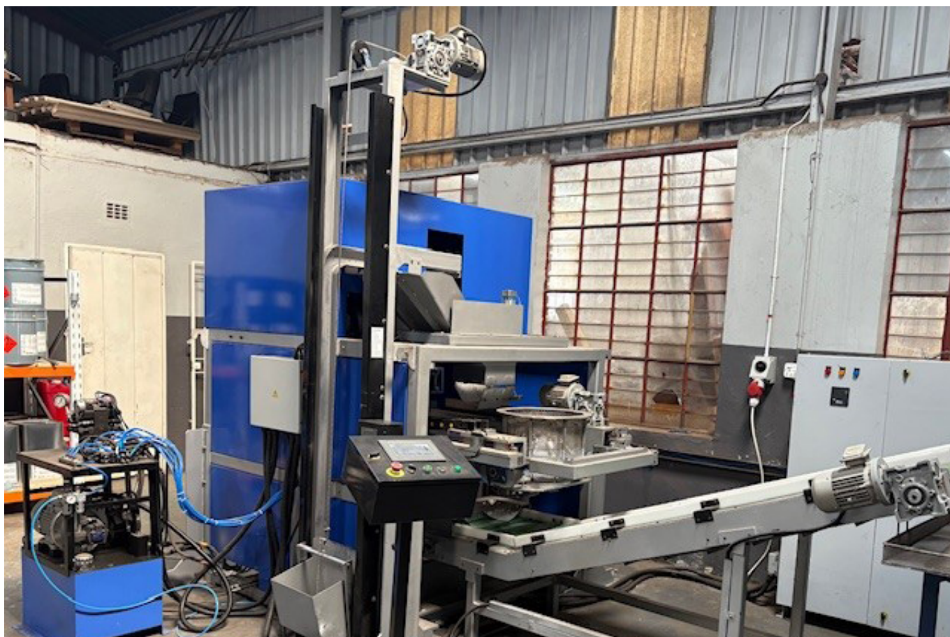
Zinc flake coating machine. “We have recently installed an automated zinc flake coating machine. Zinc flake finishing is essentially an automotive specification type finish and one of its biggest advantages is the long and durable service life it gives finished components. Here we will be coating things like fasteners, brackets and some smaller components like springs. Our aim with installing this machine was mainly to target the automotive and mining industries. It is however not just limited to these, it can also be used in most other industries.”
