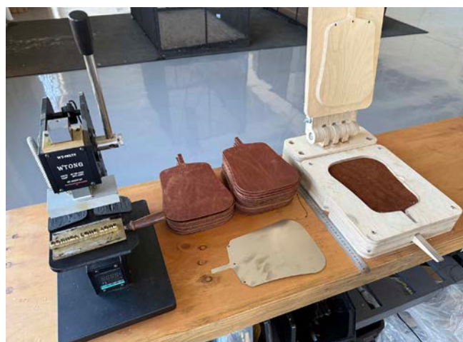
The leather cutting and sewing department has seen the addition of a multifunctional hot stamping machine for providing finishes to their leather products
