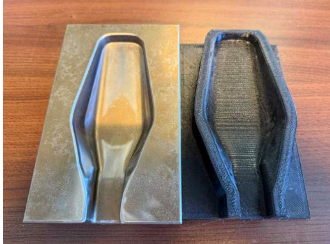
Donkey Long Tong used their Prusa i3 MK3 3D printer to prototype moulds when they redesigned the moulds that press the heads for their tong heads
