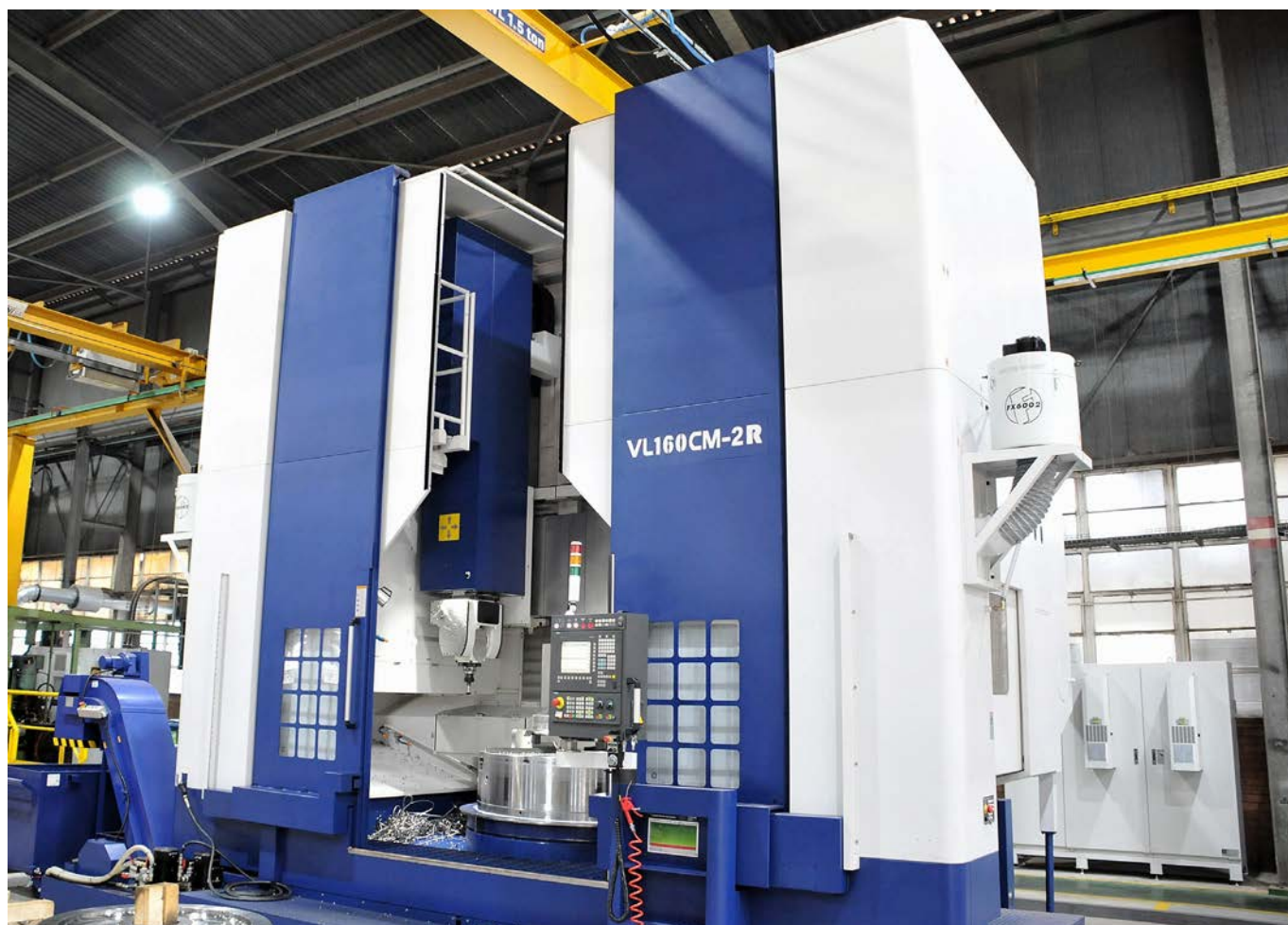
Lucchini SA have recently installed a Honor Seki VL 160CM-2R, a large, high precision, heavy duty vertical turning center with an extra wide dual vertical column that comes with live tooling. The machine has been supplied by PBS Machine Tools
