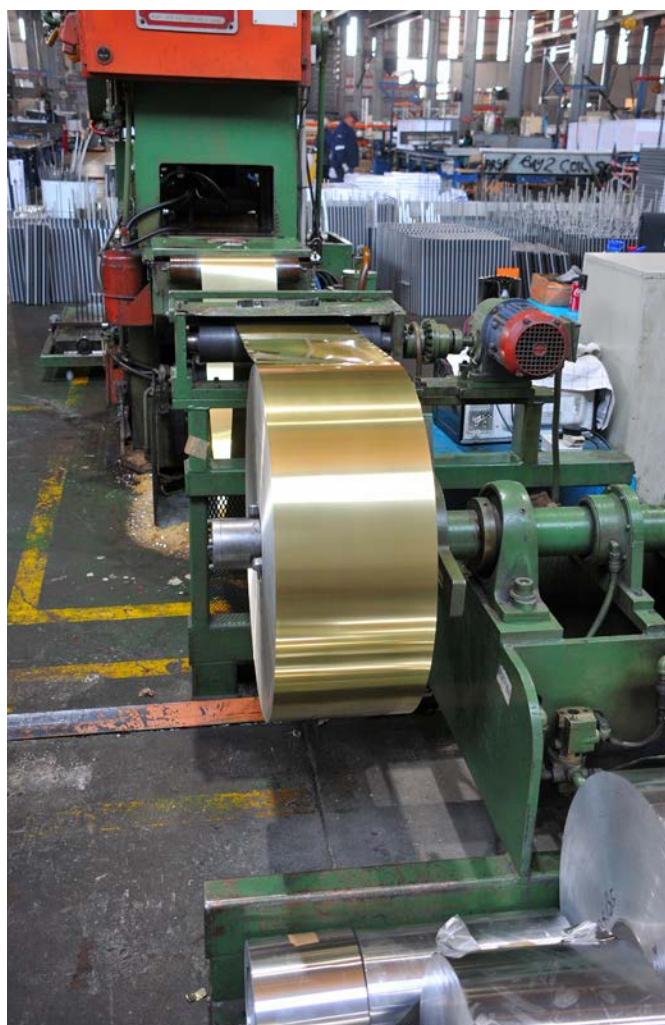
A Burr Oak Fin Press is used to stamp out the fins from rolls of foil (aluminium, polyurethane, copper or stainless steel)
