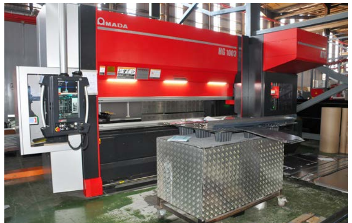
Also on the shop floor is an Amada HG 1003 ATC Press Brake with Automatic Tool Changer (ATC)
