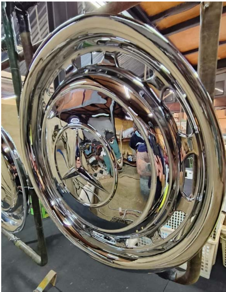
Chrome plating (bright, satin and black chrome). Chrome plating is a process that involves applying a thin layer of chromium onto a surface, typically metal, to enhance its properties. The surface of chrome plating increases wear resistance, gives a bright, shiny, and smooth finish making it easier to clean and maintain
