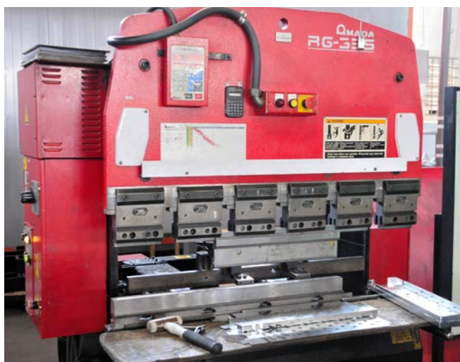
Bending work is an integral part of HC Heat Exchangers' work and the company have a number of presses including an Amada RG-35S Hydraulic CNC press brake
