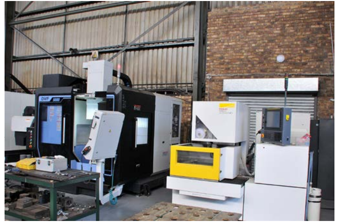
PTF have acquired their first Wire Electric Discharge Machine (EDM) – a Fanuc Robocut C400iC Wire EDM machine. It sits alongside another recent acquisition – a DN Solutions DVF 5000 5-axis mill
