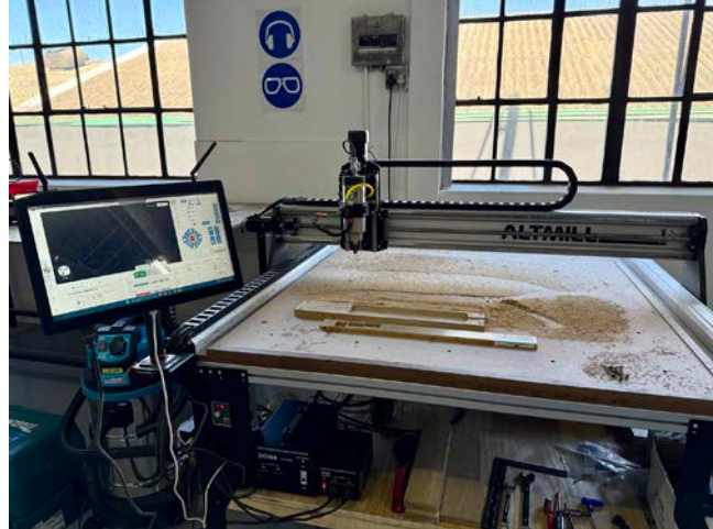
Donkey Long Tong have purchased two CNC routers to aid their woodwork department – one is for rapid prototyping and the other for full-scale production
