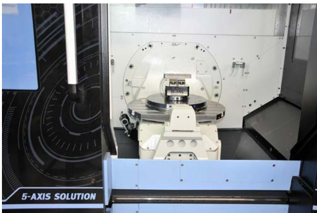
The DN Solutions DVF 5000 5-axis mill is fitted with Lang Technik fixturing
