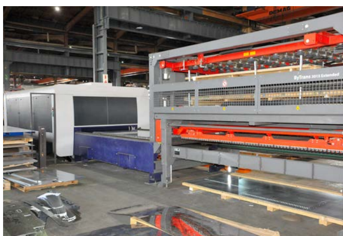
Typically, material worked with ranges from 0.5mm to 3mm but HC Heat Exchangers is able to process material up to 6mm thick. Pictured is their Bystronic 3015 6kW fiber laser with a ByTrans Extended two cassette loading system
