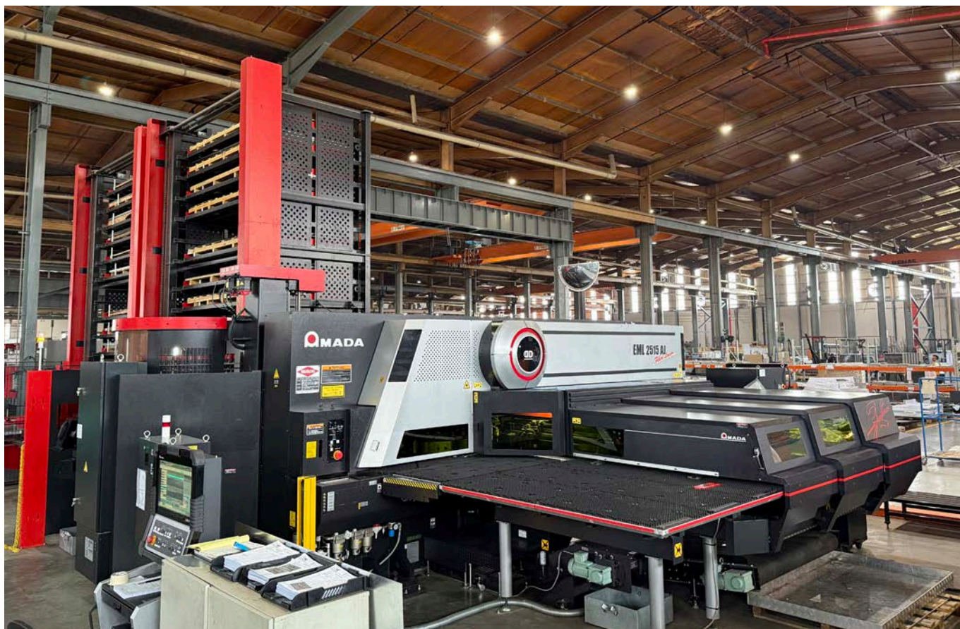
HC Heat Exchangers make use of an Amada EML 2515 AJ fiber laser / punching combination machine that processes 86 tons of thin gauge sheetmetal a month on average. That's about 2 400 sheets or 8 800m 2 of sheetmetal. The machine is equipped with two 10-tower loading and unloading pallet changers and an automatic turret tool changer
