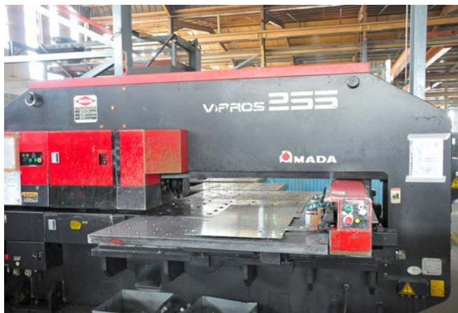
Built to last, HC Heat Exchangers also make use of an Amada Vipros 255 CNC turret punch press
